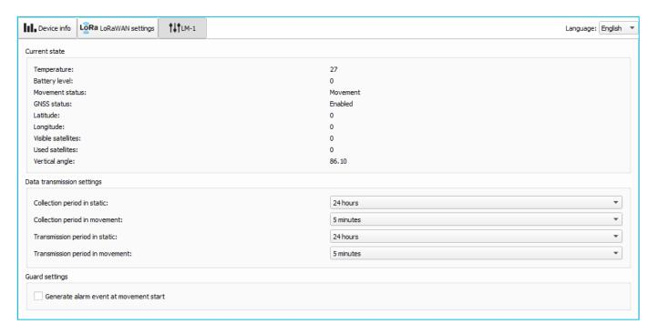
Current state – displays the current parameters of the device - the temperature, the battery level, the accelerometer and GNSS module states, latitude and longitude, the number of visible and used satellites and the angel of deviation from the vertical.
